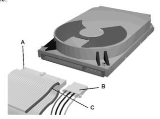
Figure 4 - 29 : Cabling an IDE Hard Disk Drive
